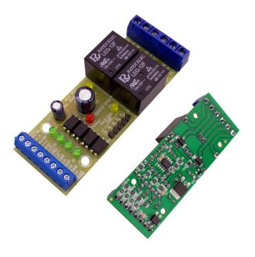
This device is a custom reprogrammable controller on the base of microcontroller PIC12F1572-I/SN with digital inputs and relay outputs.
