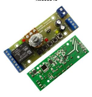
The device is constructed on the base of modern microcontroller and it is destined for controlling of driver for unipolar or bipolar stepper motor with controlling signals STEP and DIR.
