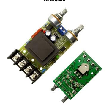
The device is based on a modern microcontroller and destined to a regulator of speed for a drill, a fan, a lighting regulator, a heater and other consumers supplied with power voltage to 230V.
