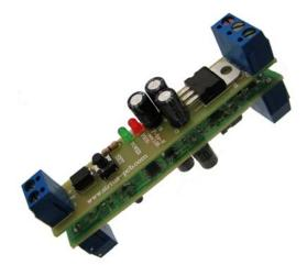
The device is used for converting of frequency in to power supply voltage, it finds its destination in industry in controlling of frequency invertors etc. It is constructed on the base of the microcontroller PIC16F1705 I/SL.
