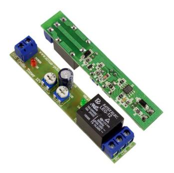
The device is used for automatisation of cyclic industrial processes with adjustable period of time for play mode and for pause. The Timer starts with supp;ying of power supply voltage. Relay output has NO (normally open), NC (normally closed) and COM (common) terminal for powering on of load.
