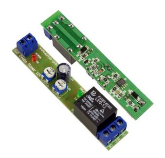
The device is used for automatisation of cyclic industrial processes with adjustable period of time for play mode and for pause. The Timer starts with powering on power supply voltage. Relay output has NO (normally open), NC (normally closed) and COM (common) terminal for powering on of load
