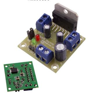
The device consists in two-channel bridge audio amplifier constructed on the base of integral scheme TDA7375. The specifications of the device are: protection from grid noise, good sound, without a need of preamplifier, unipolar power supply, suitable for accumulator of 12V and easy for assembling.
