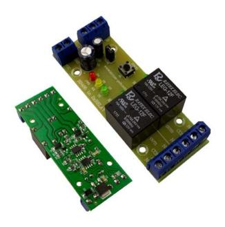
The device is commonly used for relay control through RS485 communication interface, standard MODBUS RTU or simplified protocol.
