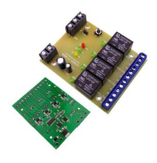
The device is commonly used for relay control through RS485 communication interface, standard MODBUS RTU or simplified protocol.
