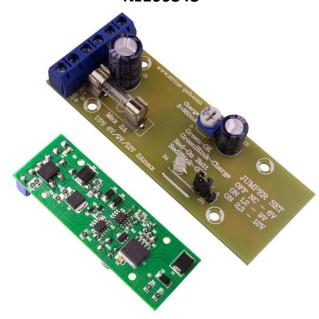
The device is based on contemporary microcontroller and it is an uninterruptible power supply (UPS) for voltage of 6V, 9V, 12V.
