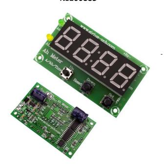
The device is based on contemporary microcontroller and is applicable for measurements of electric current (A) and electricity (Ah). Ah Meter is commonly used in electrochemical systems such as galvanization, battery capacity measurement and etc.
