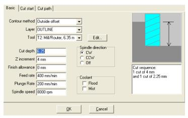
We want to cut around the outside so we use an outside offset. For the layer select 'OUTLINE' as this is the profile we want to cut. The layers 'TEXT' and 'OUTLINE' were created in the original drawing. See your CAD package documentation on how to create layers.
