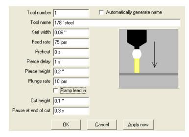
Enter 1 in the tool number. Tools are always displayed in numerical order so the tool number can be used to group different tool settings. Turn off 'Automatically generate name' and enter a name for this tool. You can have a library of tool definitions for different thicknesses of material, machine settings etc.
