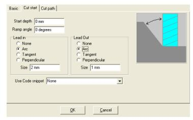
Click on the 'Cut start' tab and set 'lead in' to 'Arc' and enter 5mm for the size. The cutter will now plunge in 5mm from the start point then enter the profile smoothly without leaving any marks. You can do the same for the lead out.
