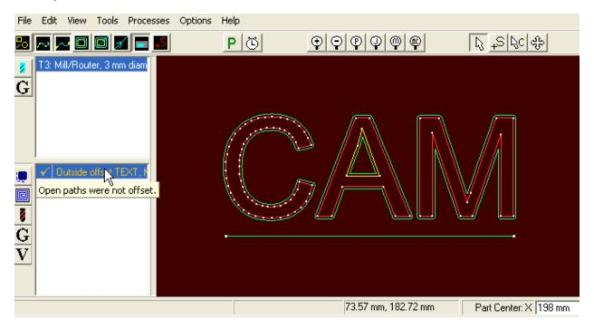
Experiment with the 'Show toolpaths' , 'Show rapid moves' and 'Show path directions' buttons to see what effect they have on the display.
