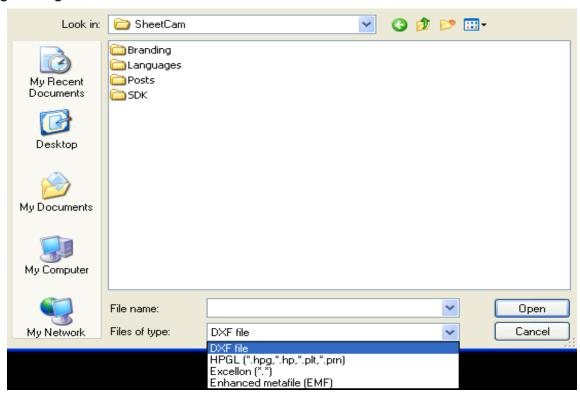
Selecting 'Open drawing' from the 'File' menu opens a pop-up window allowing you to browse for your drawing file. Acceptable formats are DXF, HPGL, Excellon or EMF files. The formats are selectable from the drop down menu. Each particular format will open its own specific settings dialogue window when you select the file and click on **<Open>**.
