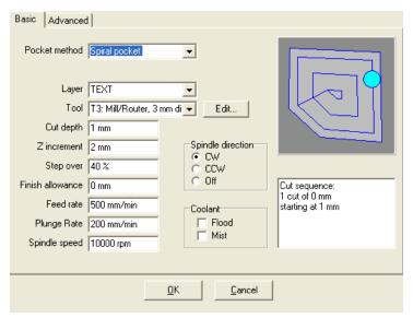
In 'Pocket method' select 'Spiral pocket'. For the layer select 'TEXT'. In the main window the text and the box around it is highlighted in white to show the parts of the drawing that are going to be used by this process.
