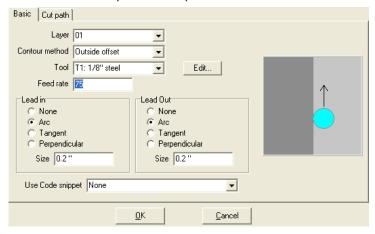
Select the '01' layer in the 'Layer' drop down list. We want to cut the part out of the sheet so select 'Outside offset' in the 'Contour method' box. Select 'Tool 1' in the 'Tool' list. Doing this sets most of the parameters from the tool definition we did earlier.
