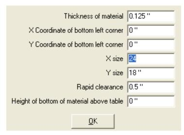
We will be cutting this sign out of a 2' x 18" off-cut of 1/8" sheet. The sheet will be placed up against the 0,0 datum bar.
