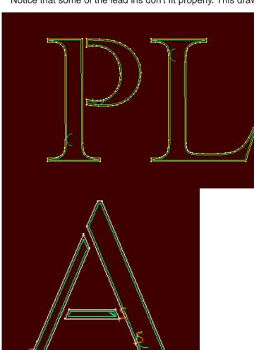
Click on the 'Place cut start point' button S. Each start point is marked with a red 'S'. Start points can be placed on any junction between lines/arcs (a segment end). If you have the show segment ends button down you will see these points marked with white dots. The cursor changes to an arrow with an 'S' when it is near a segment end.
