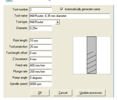
Remember that as soon as you leave the diameter box the diameter will be converted to millimetres. Now click on **<OK>** to save the settings.
