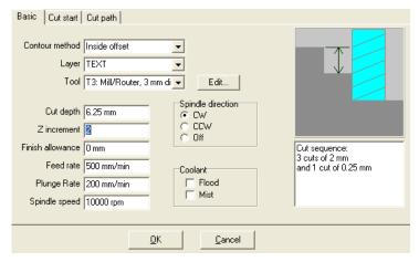
We want to cut the letters out of the sheet so select 'Outside offset' in the contour method box. Select the 'TEXT' layer in the 'Layer' drop down list. Select tool 3 in the 'Tool' list. Doing this sets most of the parameters from the tool definition we did earlier.
