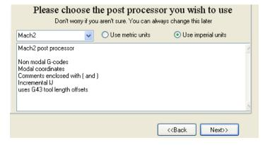
Select the correct processor for your machine controller. A brief description of the processor file will appear in the lower window (if available).
