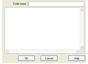
New code snippet creates a 'tool' that consists of one or more lines of G-code. This is then used by the 'Insert code' process.
