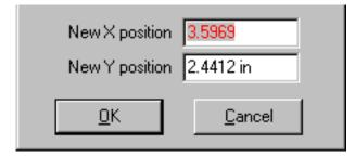
Enter the actual coordinates of this point and click **<OK>.** Now click on the second point on the part in the view window and enter the coordinates of that point and click **<OK>.** The drawing will be moved and rotated to suit 'the job'.
