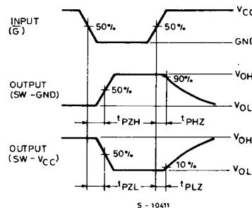
NOTE: SUCH A LOGIC LEVEL SHALL BE APPLIED TO EACH INPUT THAT THE OUTPUT VOLTAGE STAYS IN THE APPPOSITE SIDE TO THE SWITCH CONNECTION LEVEL, WHEN THE OUTPUT IS ENABLE
