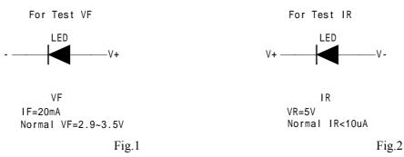
c. The reverse voltage mustn't exceed 5v when lighting on or testing the LED, otherwise, the leds will be damaged.
