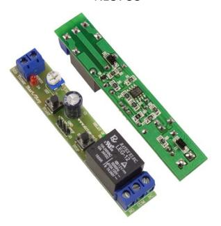
The device is intended to power off electrical currents operating on direct or alternating current after a predetermined period of time. The Timer is with a relay output with normally open (NO), normally closed (NC) and common (COM) terminal. Operational range 0.5 seconds to 490 seconds.
